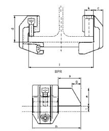
Can be used with S 235 parallel flanged beams (free fom oil and grease) and for trolleys with a max. travel speed of 36 m/min.
